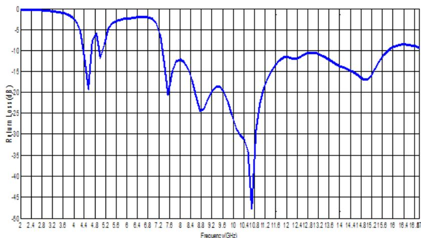
Fig.4: Return Loss for I slot patch antenna
