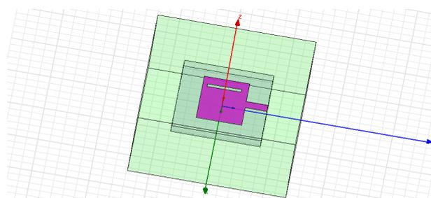
Fig.1: Rectangular patch antenna with I slot
