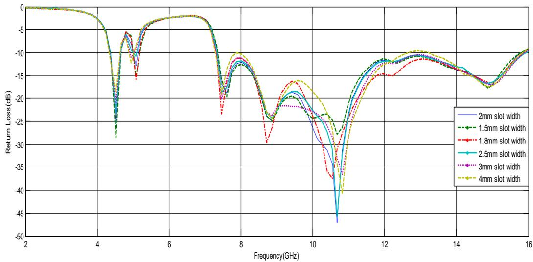
Fig.2: Return Loss with Variation in Slot Width
