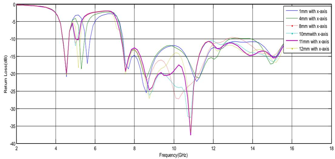
Fig.3: Return Loss with Variation in Slot Position
