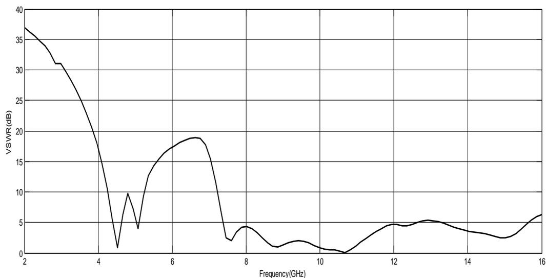
Fig.6: VSWR for I Slot patch antenna
