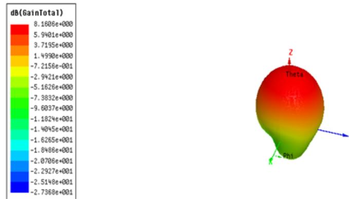
Fig.5: Gain Total for I slot patch antenna
